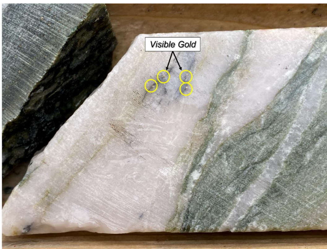
Figure 1. Specks of visible gold in hole BF21-19 drilled at the Black Fly Northeast Zone. BQTK core of a diameter of 40.7 mm.
