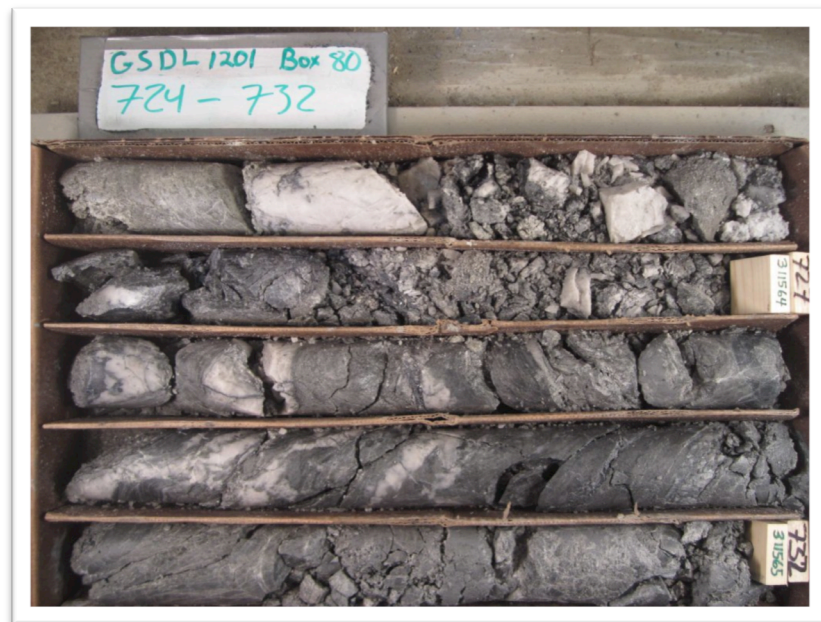
Intense Brecciation and Fractured Schist hosted Stockwork – GSDL 12-01 Figure 7.2.3D
