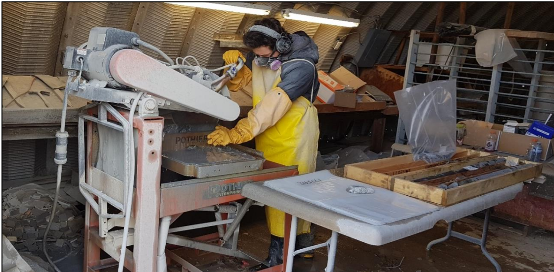
Figure 12.3 Drill Core Cutting at Sampling at Silver Hart Core Storage Facility
