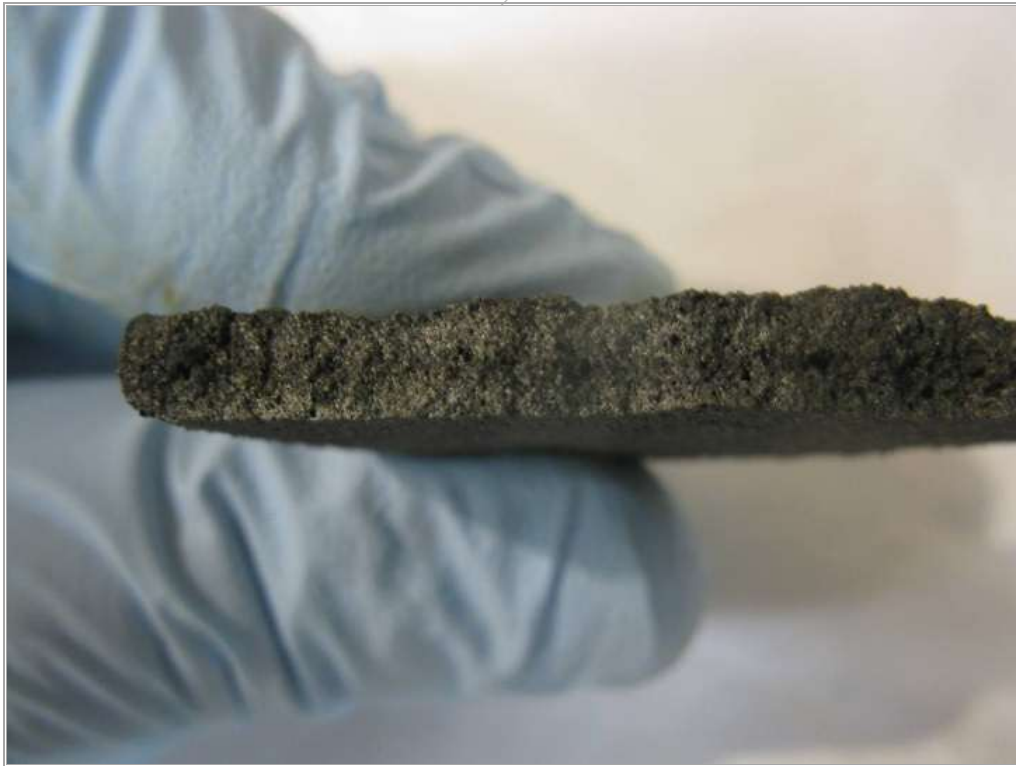
Figure 13-20: Roasted Calcine after the Phase II Test for 30 minutes at 650°C
