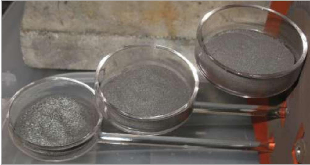
Figure 13-19: Roasted Calcine in Three Trays from the Phase II Test at 650°C
