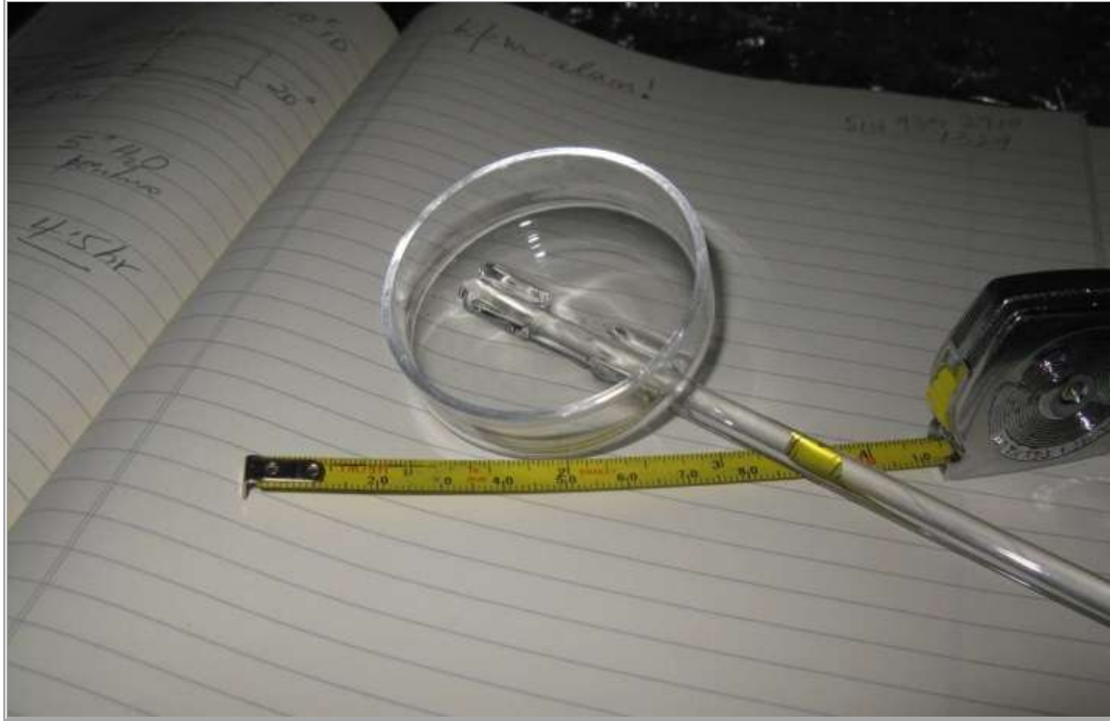
Figure 13-15: Test Tray Used to Contain Concentrate Sample for Roasting Testwork
