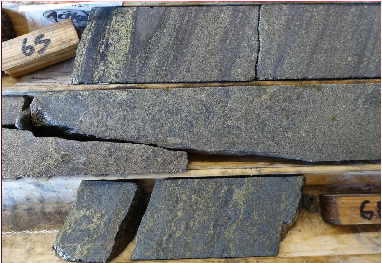
Figure 18 : Mineralization in hole CLDD22-02 at 65 m showing mostly stratified pyrite, chalcopyrite and sphalerite. The hole returned 3.9% Cu & 0.49% Zn from 65.15 to 68.3 m. Core is NQ, 4.7 cm in diameter. Photo AC, September, 2024.
