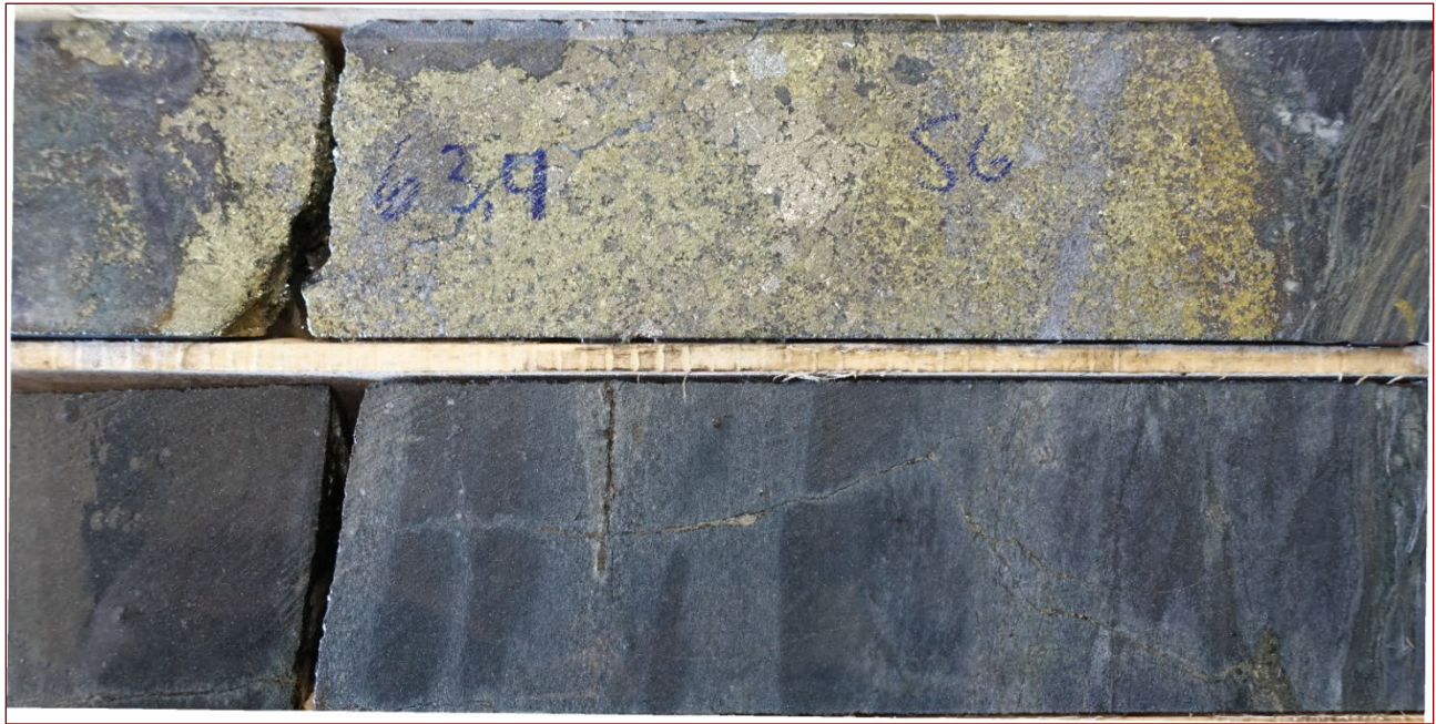
Figure 19 : Mineralization in hole CLDD23-07 at 63.4 m showing mostly massive chalcopyrite and pyrite within quartz-rich layers and siltstone sequences. The hole returned 6.63% Cu from 63.32 to 63.62 m. Core is NQ, 4.7 cm in diameter. Photo AC, Sept 2024.
