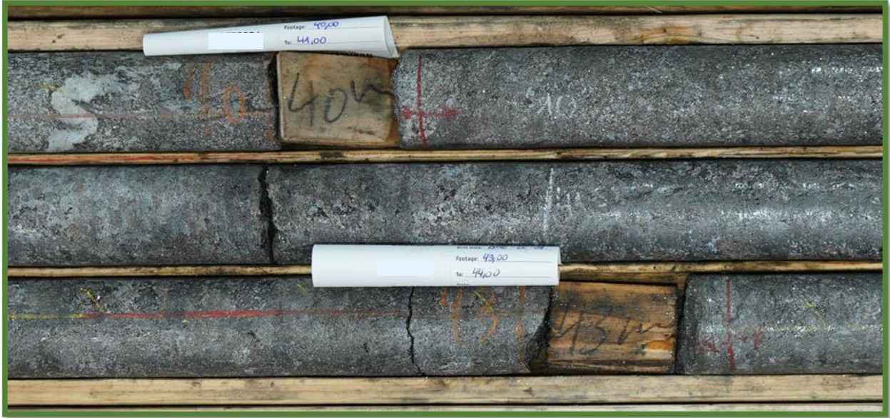
Figure 5: Drill Core from BK-22-21, A) Graphite enriched zone from 35.6 to 52.2 (16.6m length), B) inset; a selected example of coarse flake graphite enrichment encountered between 40 – 43 m.
