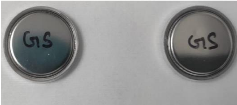
Figure #1 Graphene Lithium Ion coil cell batteries made out of Green Battery graphite
