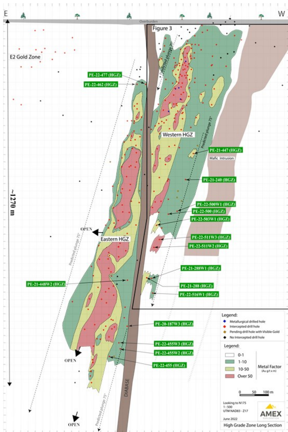
Figure 2: Longitudinal section of the High Grade Zone, with today's released hole locations in green labels. Assay results are presented in core length (m). True width is approximately 45-70% of reported intercepts. Metal factor is defined as gold grade in grams per ton multiplied by core length in metres.
