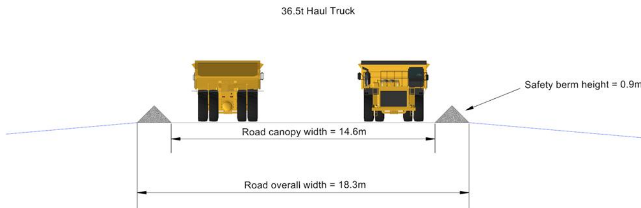
Figure 16–30 : Double Lane road design
