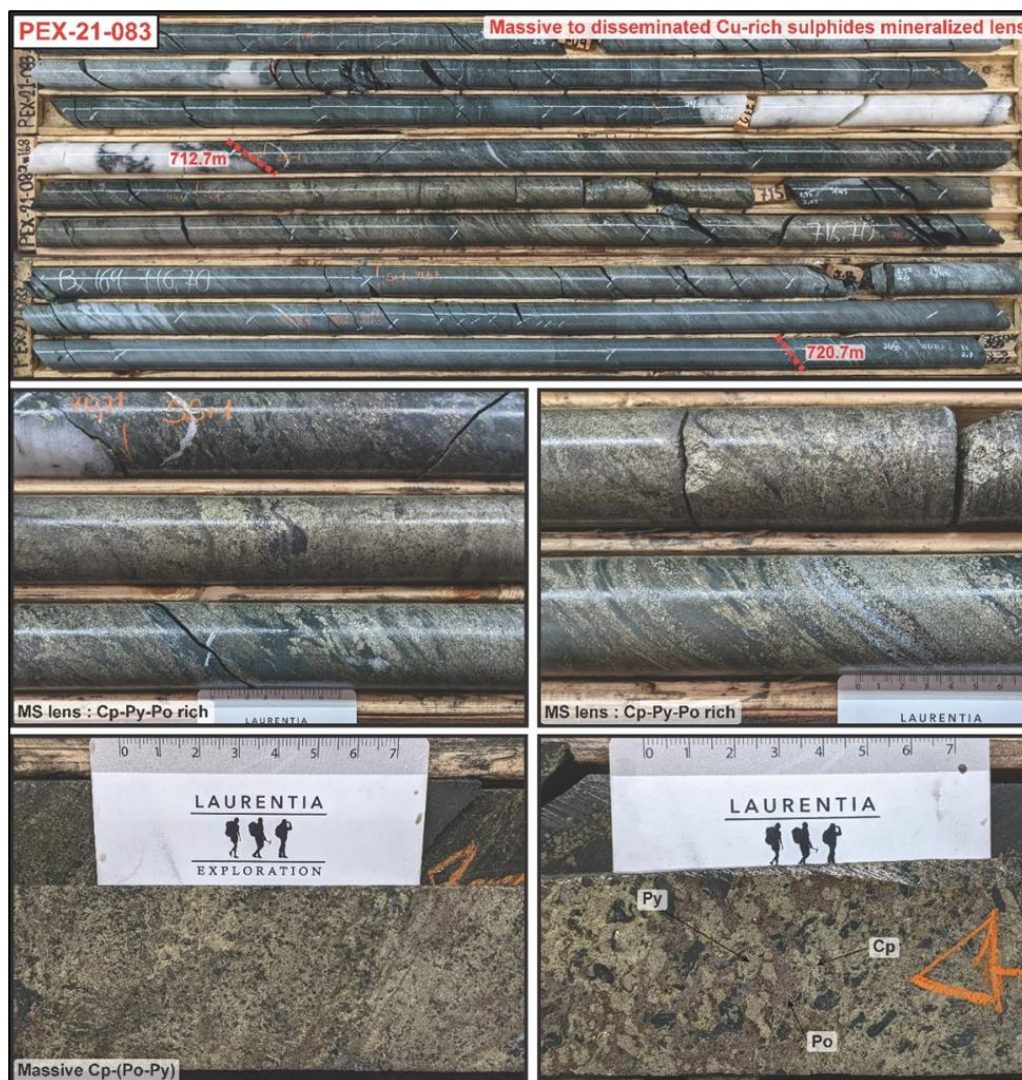
Figure 7–10: Photographs of the Massive to Disseminated Sulphide Cu-Rich Lenses of the QF Zone Intersected in Drill Hole PEX-21-083
