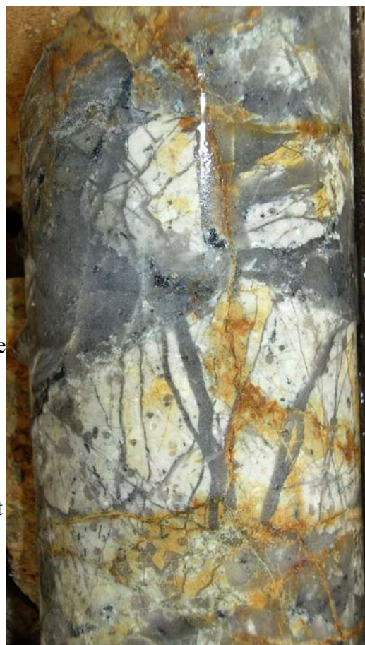
Figure 2: Intense brecciation textures at approx 100m in DDH06-43.
