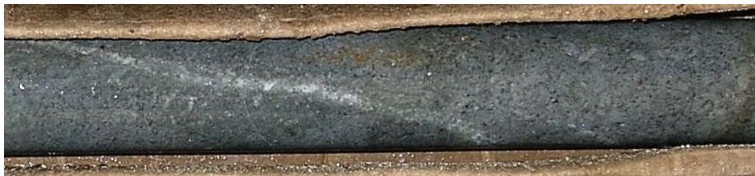
Figure 3: Gold bearing latite sill in DDH 06-45 at 201m. Logged as lgi - light grey intrusive.
