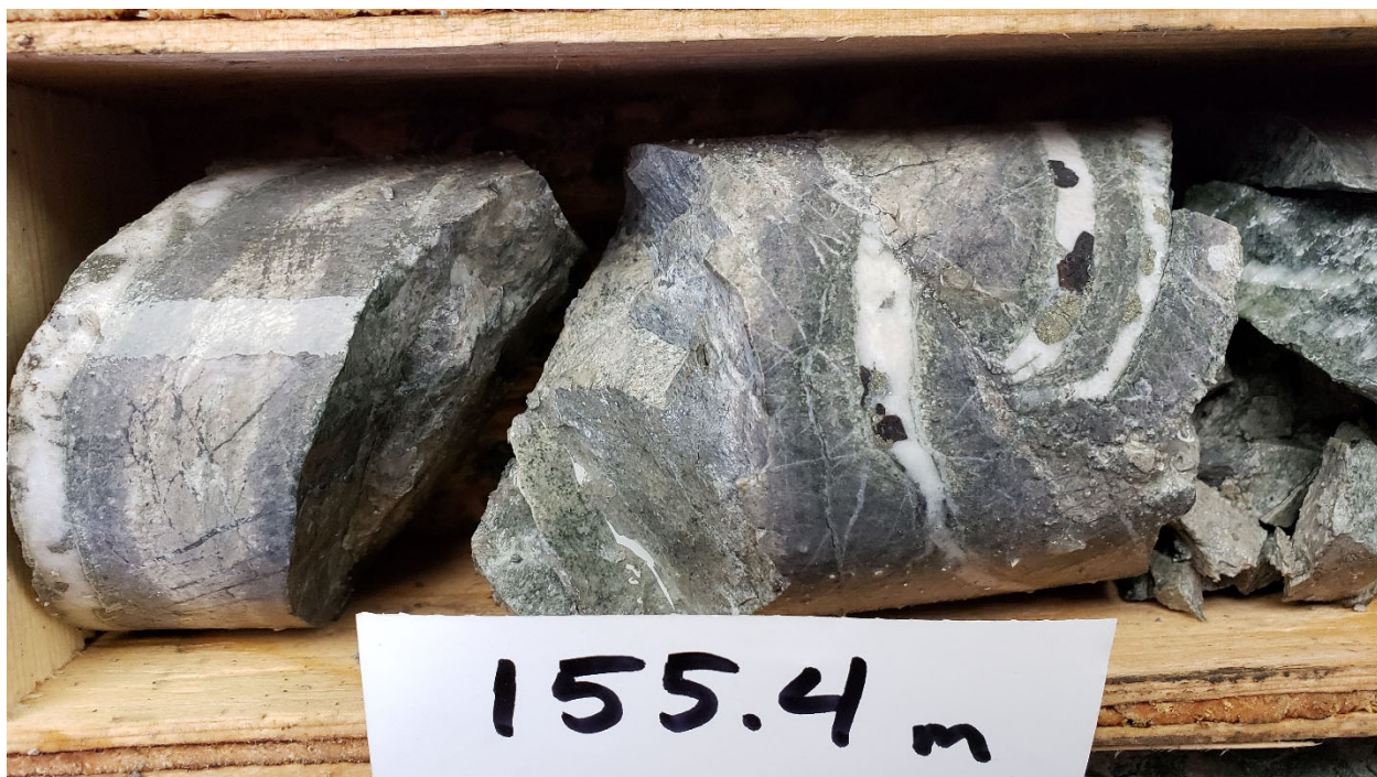
Figure 4 – Strongly silicified, sericitized and stockwork-veined section from Hole APR-18 grading 2.27 g/t Au and 15.9 g/t Ag over 0.5 metres.
