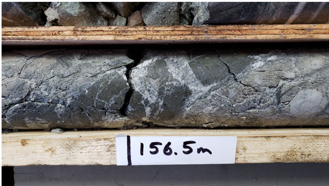
Figure 3 – Strongly sericitized, sulphidized and brecciated section from Hole APR-18 grading 5.91 g/t Au and 7.1 g/t Ag over 0.8 metres
