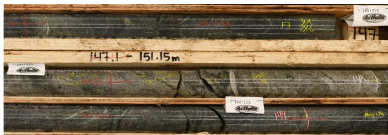
Photo 2 – Typical sheared and mineralized diorite from Hole 068 on the Blue Sky trend. The 1.15 m interval from 147.05 to 148.20 m averaged 4.94 g/t Au.
