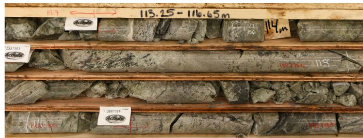
Photo 1 – Sheared and mineralized andesitic ash tuff from the Thunder North zone, Hole 072. Note the characteristic spotted to wormy pyrite “disease” alteration. The 0.95 m interval from 115.20 to 116.15 m averaged 237 g/t (6.91 oz/ton) Au.
