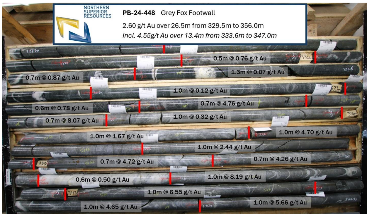
Figure 10: PB-24-448 – Grey Fox Footwall core picture with assay results – part 1
