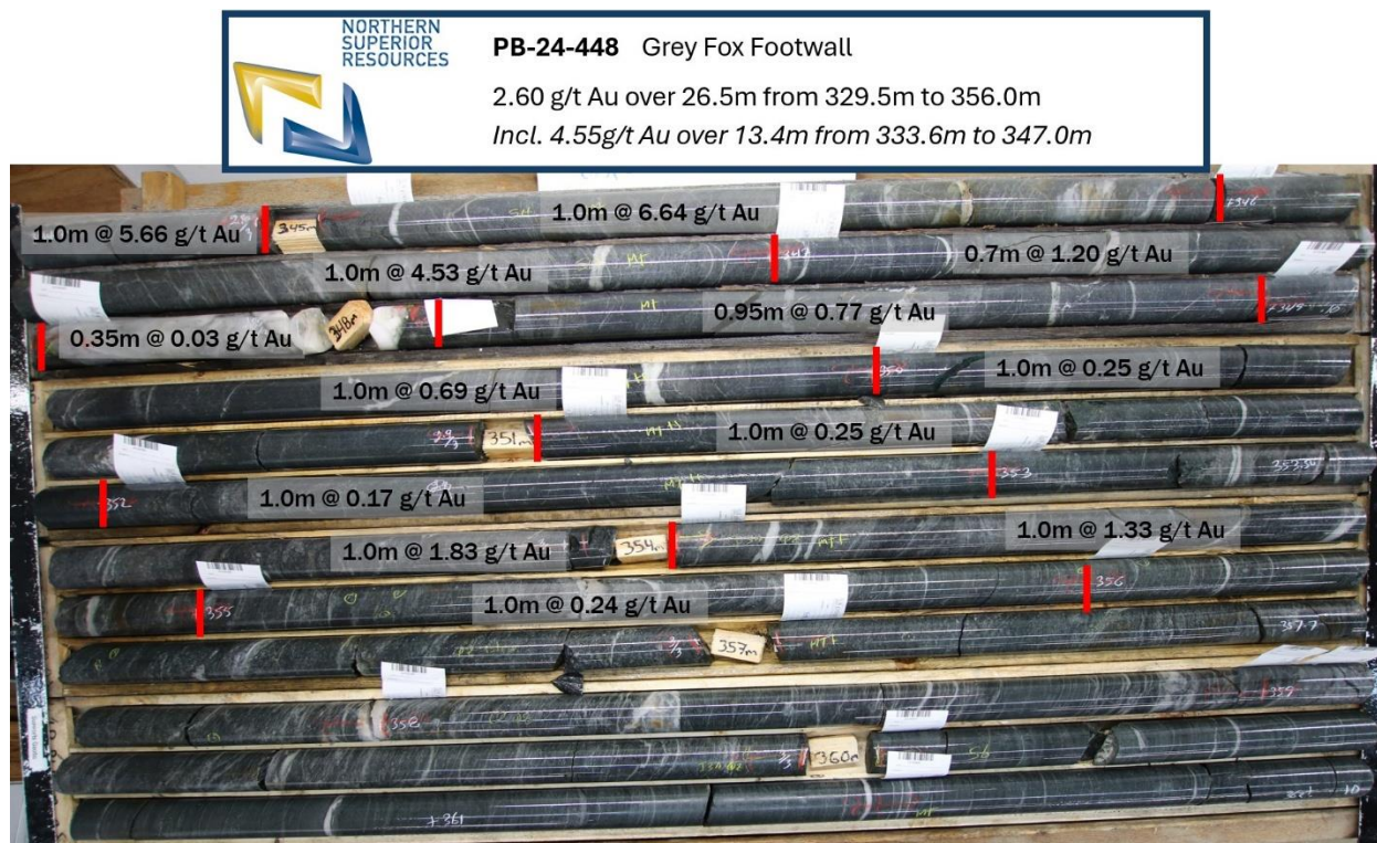
Figure 11: PB-24-448 – Grey Fox Footwall core picture with assay results – part 2
