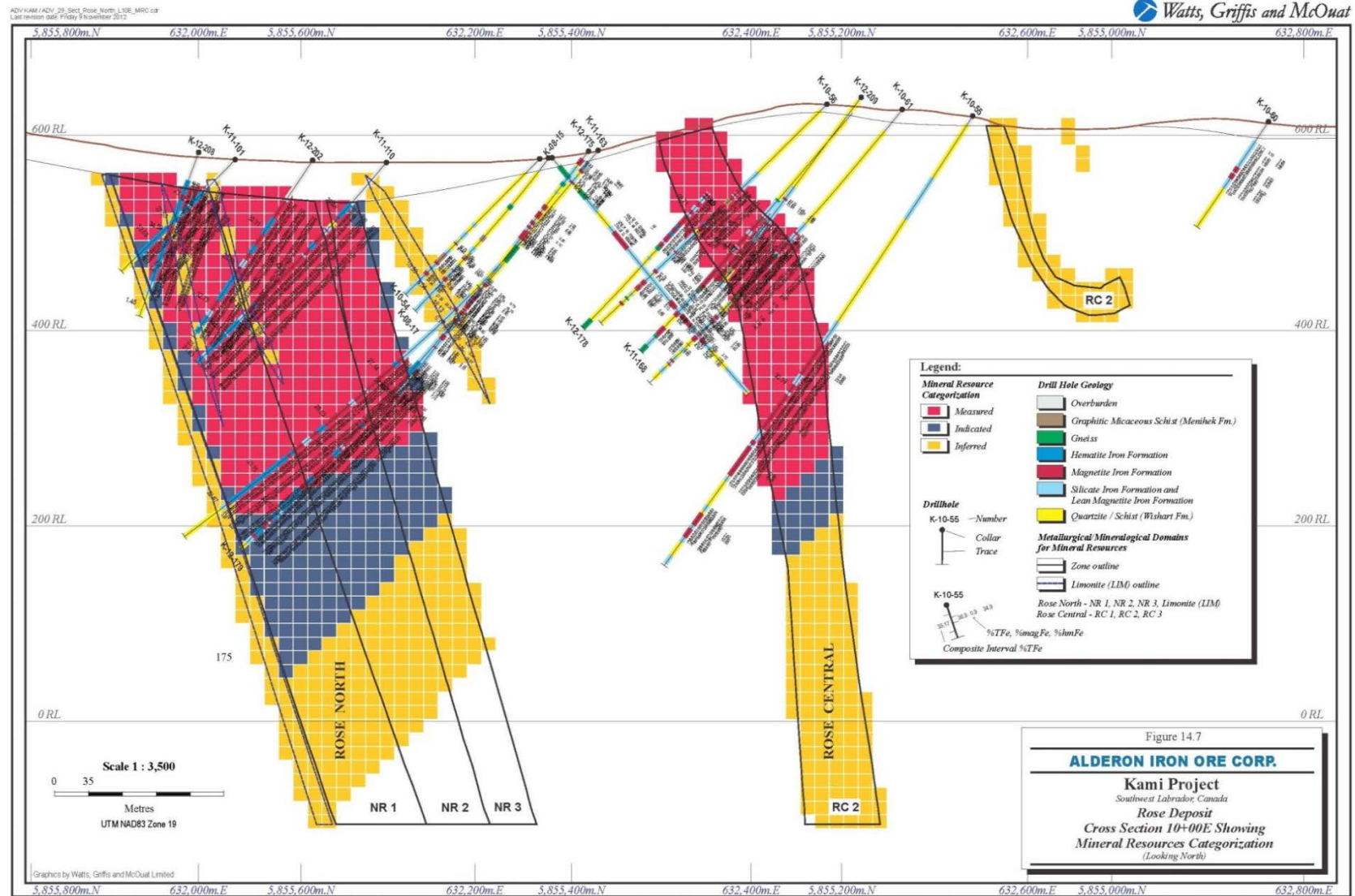
Figure 14-7: Rose Deposit Cross Section 10+00E Showing Mineral Resource Categorization
