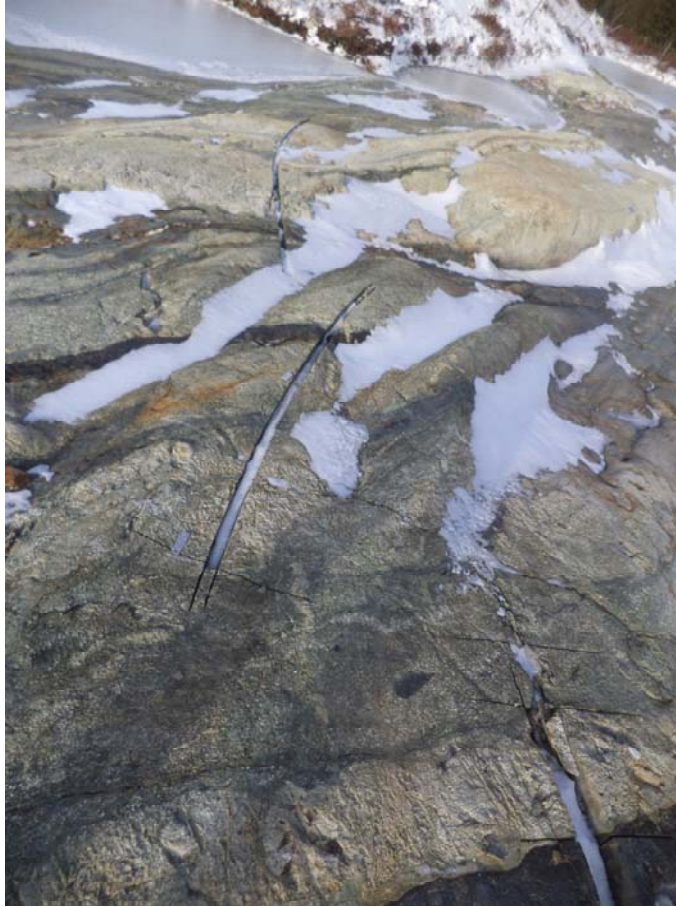
Picture 15: View of the sampling channel on the broad stripping excavated on Lac Doré North. Notice the uniform width of the channels, but also their swirling attitude.
