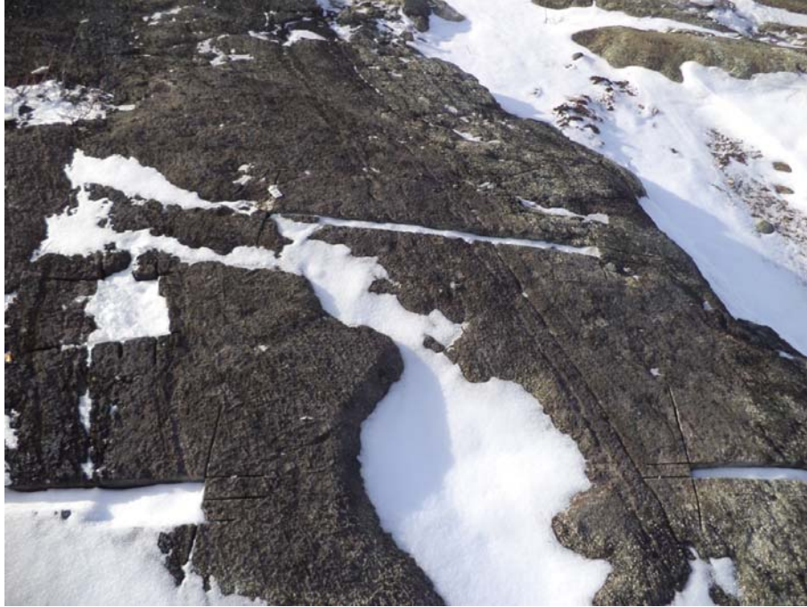
Picture 16: Channel sampling of a magnetite rich layer on Lac Doré North stripping. Notice the discontinuous channels with gaps between segments.
