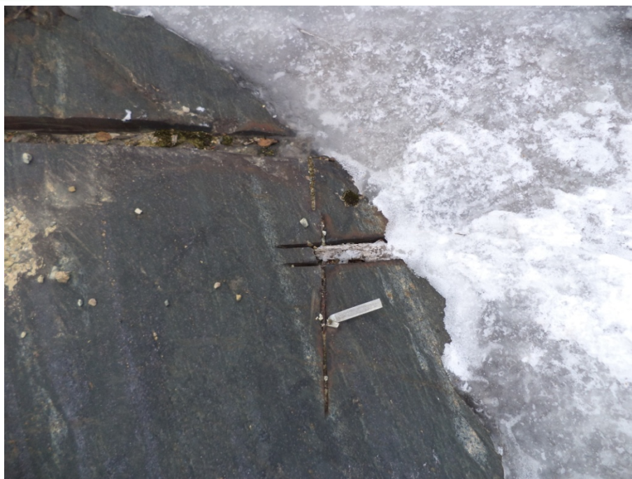
Picture 18: Recent view, taken by the author in the course of his mandatory field visit, of the channel sampling carried out by McKenzie Bay in 1997. Notice the absence of gaps between samples and that sampling tags are still in place.
