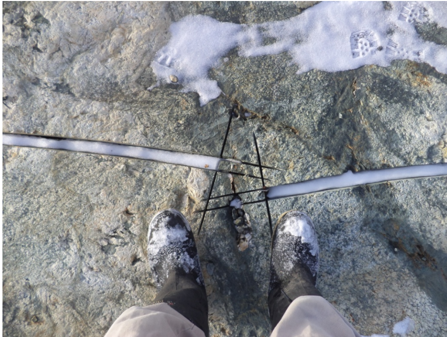
Picture 17: Channel sampling of a barren anorthosite, showing gaps left between samples.
