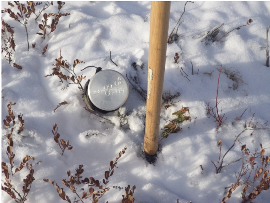
Picture 20: View of the capped casing found at LDN-09-04 site.
