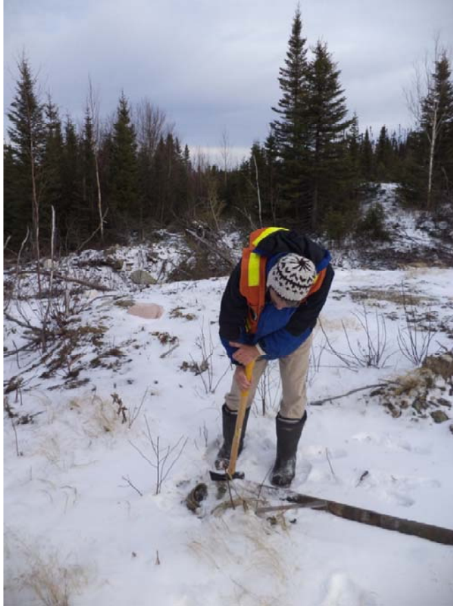
Picture 24: View of the casing, cut at a bevelled angle, as left at LD-13-02 drill hole.
