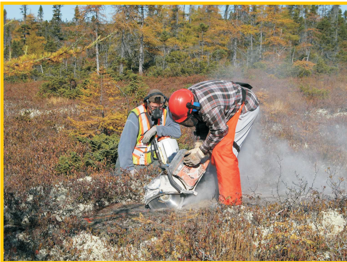
Figure 23b. Channel cutting with a gas-powered diamond saw. UTM Coord; Easting: 549003; Northing: 5571849 (NAD83; Zone 20N).
