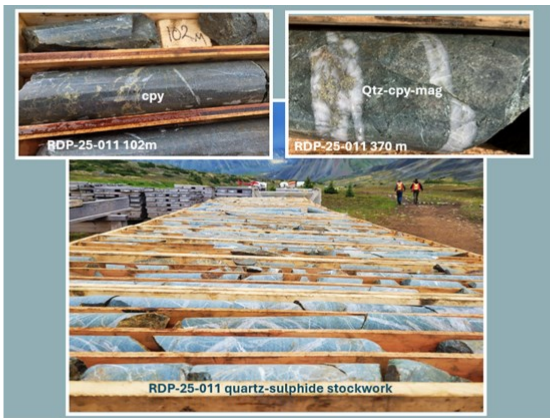
Figure 5 RDP-25-011 Drill Photos
