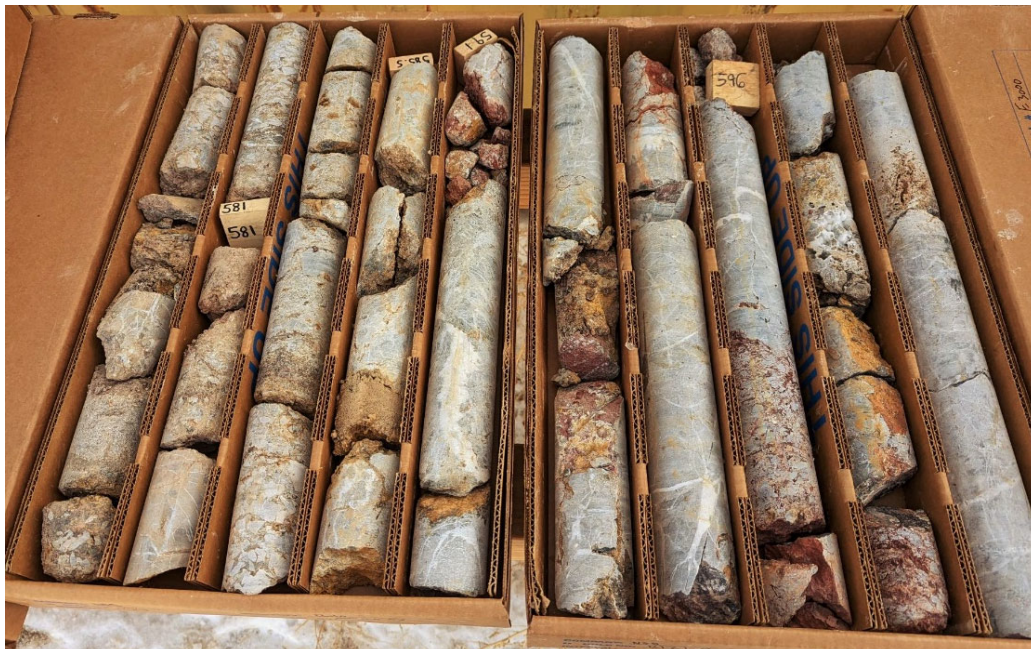
Drill core from drill hole BL21-01 showing mineralized, decalcified, silicified, and brecciated interpreted Windfall Formation within South Mine Fault Zone (~579-599 ft.)
