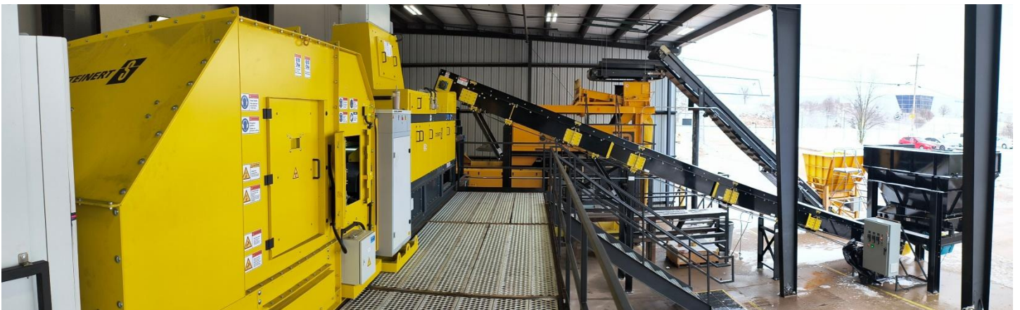
Figure 5: Steinert Sensor-Based Ore Sorting Machine
