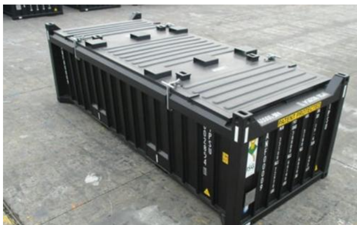
Fig. 7: “Rotainer” type Ore Container
