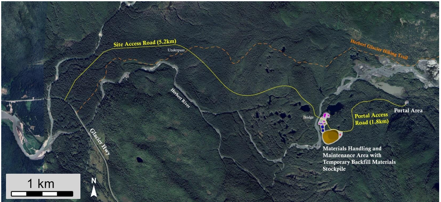
Figure 4: Conceptual Surface Infrastructure Layout Utilized for the PEA. Layout may change pending further environmental baseline studies, engineering, environmental review and permitting processes.
