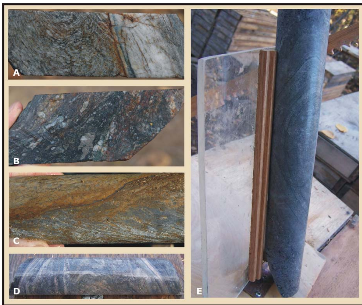
Figure 7. Examples of fold relations observed in core. A) Gneiss (left) - schist (right) contact showing a drag fold along a clear narrow tectonic contact; LM-06-13. B) Clear fold nose and apparent folded pyrite clast in graphitic quartzite breccia; contains 5.3 g/t Au; LM-06-29. C) tectonic contact between different schist units D) fold noses in core indicate the presence of fold axes nearly perpendicular to core axes E) This stick of core is correctly oriented in an orienting jig and shows a gently west-dipping nearly subhorizontal fold axis. Photos D and E courtesy of Ed Hunter.
