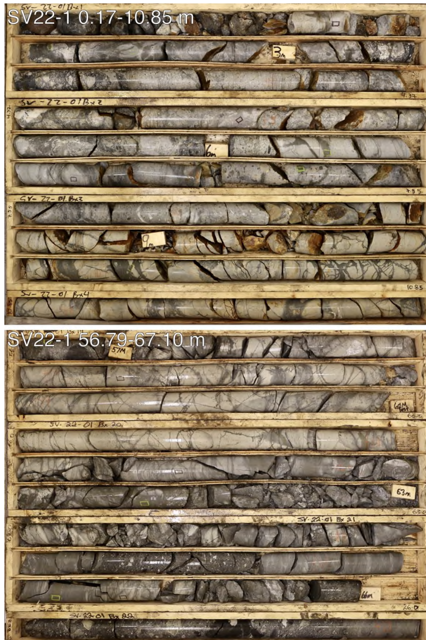
(Figure 5: Representative intervals of replacement-style sulfide mineralization in SV22-1. This type of mineralization is ubiquitous from 1.0-80.0 and 100.0-113.0 m. In addition to sulfide replacement of andesite there are several intervals of volcanoclastic debris flow breccia also hosting replacement-style mineralization.)
