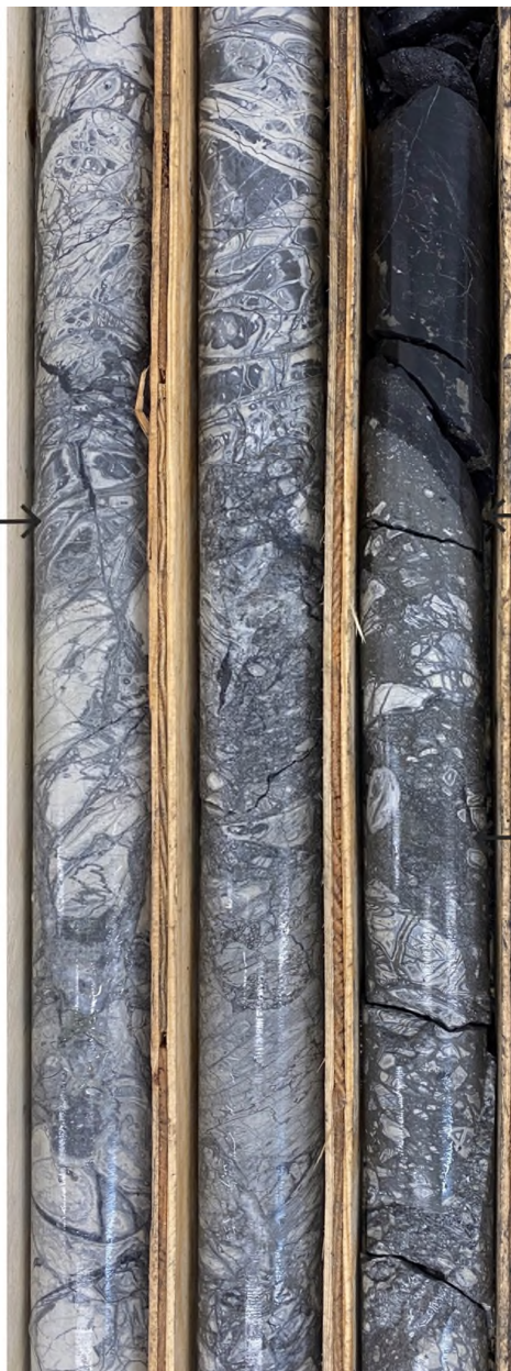
(Figure 9: SR22-4 showing intense clay alteration, silicification, and replacement-style mineralization of an andesite breccia. We interpret this as an autoclastic andesite breccia that underwent shrinkage and further brecciation during quenching of the hot lava in a submarine environment. Brecciation increased the permeability of the rock, enhancing the flow of VMS hydrothermal fluids, and creating the perfect host rock for replacement-style sulfide mineralization. Mineralization intensifies towards the contact with overlying black mudstone, with sulfide stringers emanating from the andesite breccia into the mudstone.)
