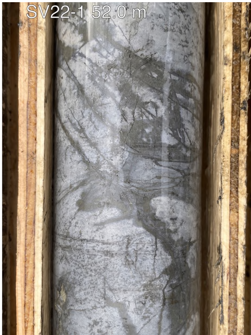
(Figure 4: Representative samples of andesite showing intense sulfide replacement from drill hole SV22-1. Andesite is intensely sericitized, corroded, and replaced with pyrite \pm sphalerite. Sulfide minerals occur as fine dendritic disseminations throughout the andesite, and within corroded fractures along with hydrothermal silica. This type of mineralization is ubiquitous from 1.0-80.0 and 100.0-113.0 m. Handheld XRF of this type of sulfide mineralization returns consistently high values of the Au pathfinder elements Ag, As, Sb, Hg and Zn. Handheld XRF cannot reliably measure Au concentrations.)
