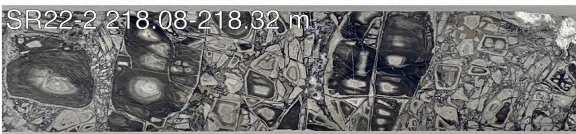
(Figure 8: Examples of intense replacement style mineralization from drill hole SR22-2. The image for 22.0-22.32 m shows intense clay alteration and sulfide replacement of coherent andesite. Perlite andesite exhibiting intense clay alteration followed by silicification and sulfide mineralization is the most common type of mineralization at Scarlet Ridge, and is represented by photos for 44.50-44.84 m and 218.08-218.32 m. Extremely intense sulfide replacement of a perlitic autoclastic andesite breccia is represented by the interval 90.00-90.33 m.)
