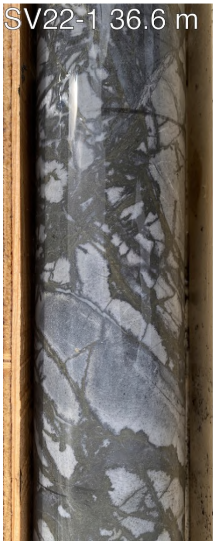
(Figure 4: Representative samples of andesite showing intense sulfide replacement from drill hole SV22-1. Andesite is intensely sericitized, corroded, and replaced with pyrite \pm sphalerite. Sulfide minerals occur as fine dendritic disseminations throughout the andesite, and within corroded fractures along with hydrothermal silica. This type of mineralization is ubiquitous from 1.0-80.0 and 100.0-113.0 m. Handheld XRF of this type of sulfide mineralization returns consistently high values of the Au pathfinder elements Ag, As, Sb, Hg and Zn. Handheld XRF cannot reliably measure Au concentrations.)
