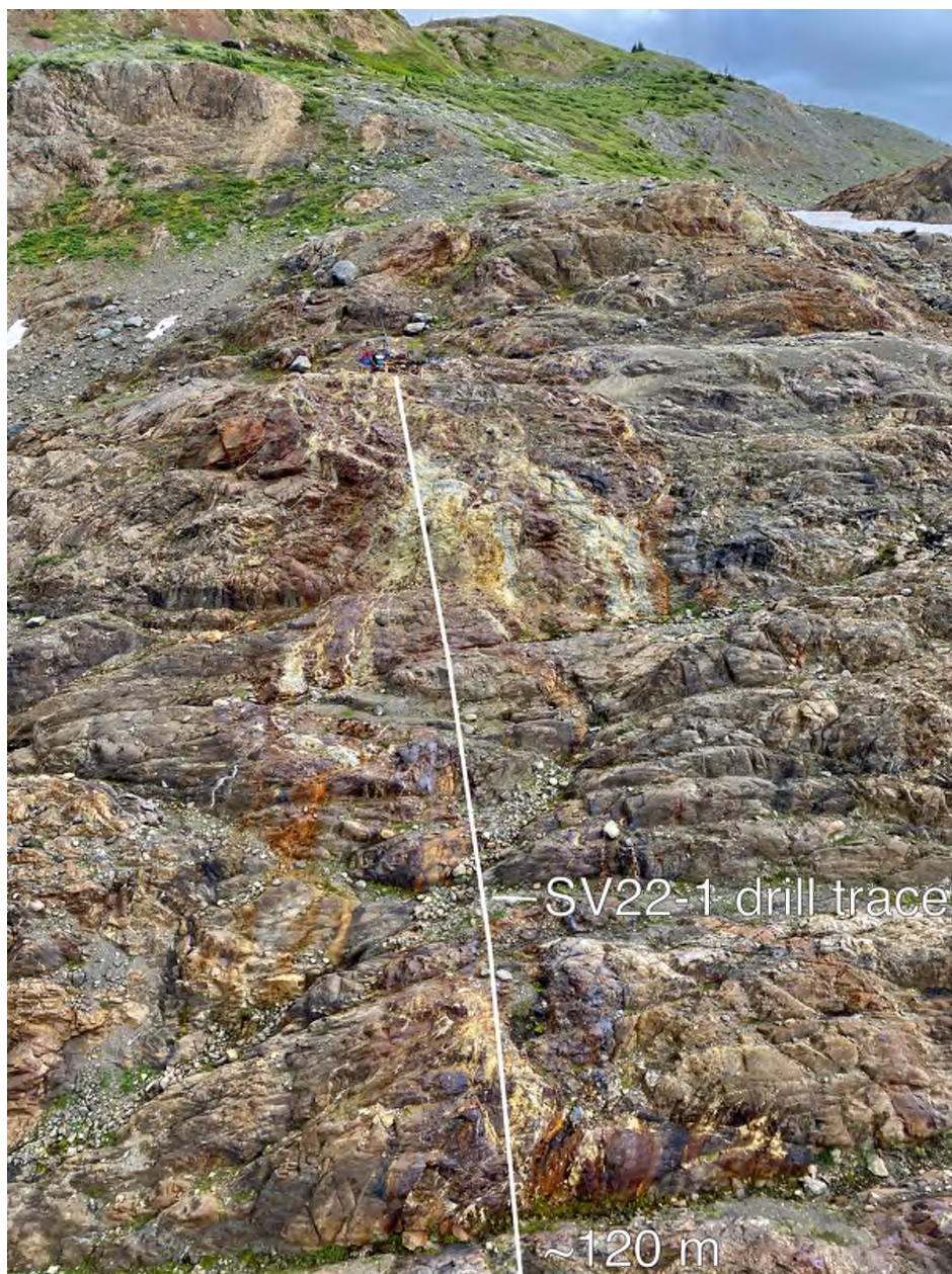
(Figure 3: The drill trace of the first 120 m of SV22-1 projected onto the surface. Intensely gossanous areas are associated with intense sulfide replacement-style mineralization. Grey patches on the outcrop are where the weathered surface has flaked off, exposing nearly complete sulfide replacement of the host andesite. Additional gossanous and mineralized rocks occur to the north (left), south (right), east (up), and west (down). Several drill holes will be drilled in 2022 to test the extent and grade of mineralization at Scarlet Valley.)
