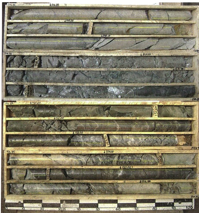
Figure 17.7 Photograph of drillhole MD 218 showing progressive deterioration of hanging wall conditions above the vein zone (Source: Exeter core photography)
