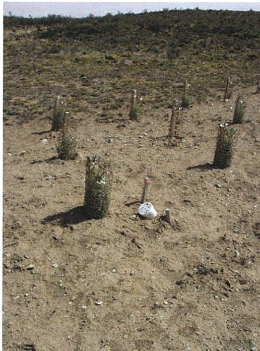
Figure 4.7 Photograph of a rehabilitated drillhole site at the Escondida prospect. The white sacks in the background contain RC chips from neighbouring drillholes awaiting removal from site (Source: Snowden site visit, 2009)
