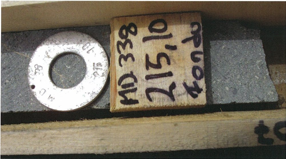
Figure 12.3 Photograph of a metal washer used as a permanent record of the drillers wooden core run markers (Source: Snowden site visit, 2009)
