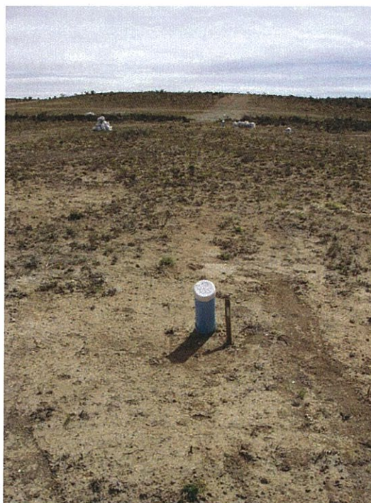
Figure 4.7 Photograph of a rehabilitated drillhole site at the Escondida prospect. The white sacks in the background contain RC chips from neighbouring drillholes awaiting removal from site (Source: Snowden site visit, 2009)
