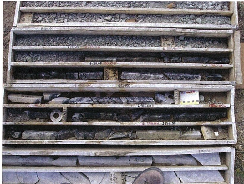
Figure 17.8 Photograph of drillhole MD 218 during the Snowden site visit showing increased hanging wall decay with time and as a result of sampling (Source: Snowden Site visit, 2009)
