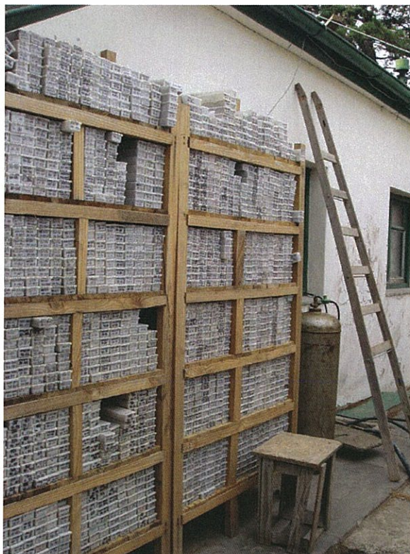
Figure 12.7 Photograph of RC chip box storage racks at Exeter's Cerro Moro base camp (Source: Snowden site visit, 2009)
