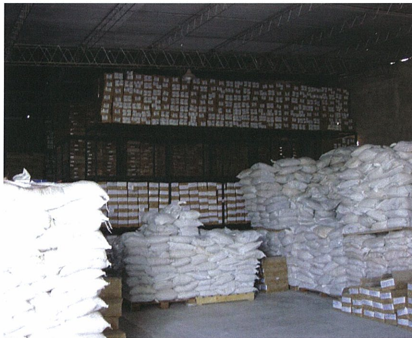
Figure 13.1 Photographs of coarse reject and reject pulp samples in storage at Exeter's Mendoza sample store (Source: Snowden site visit, 2009)
