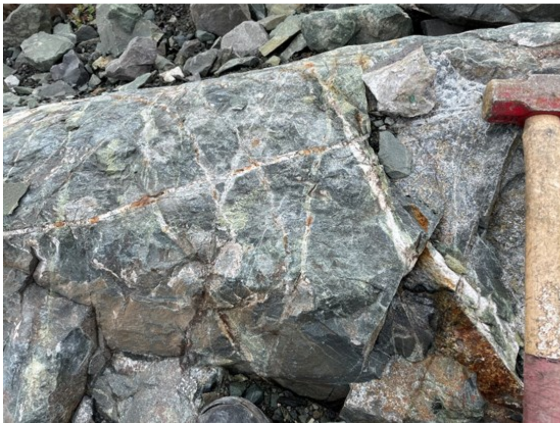
Plate 1: Example of an epidote altered, quartz-pyrite±chalcopyrite veinlet stockwork outcrop, TREK South claims. Small sledge hammer for scale.
