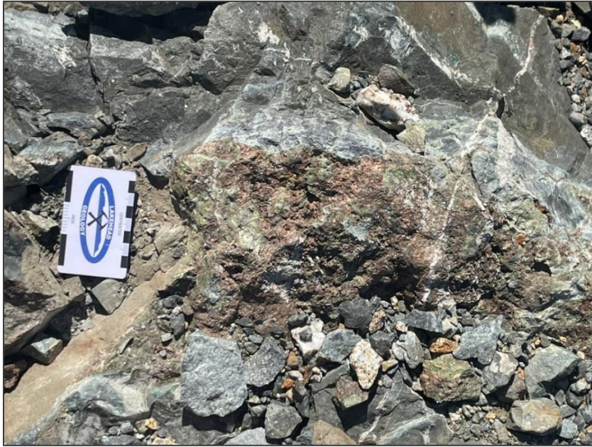
Photo 13: Well developed, relatively thick garnet-epidote skarn vein cutting andesitic volcanics at Trek South.
