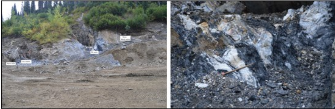
Figure 2. Working faces of the bulk sample site - September 14, 2025. Total width of photo is 40m, distance between hanging wall (right side) of 16 Vein and Pit Vein is 20m.
