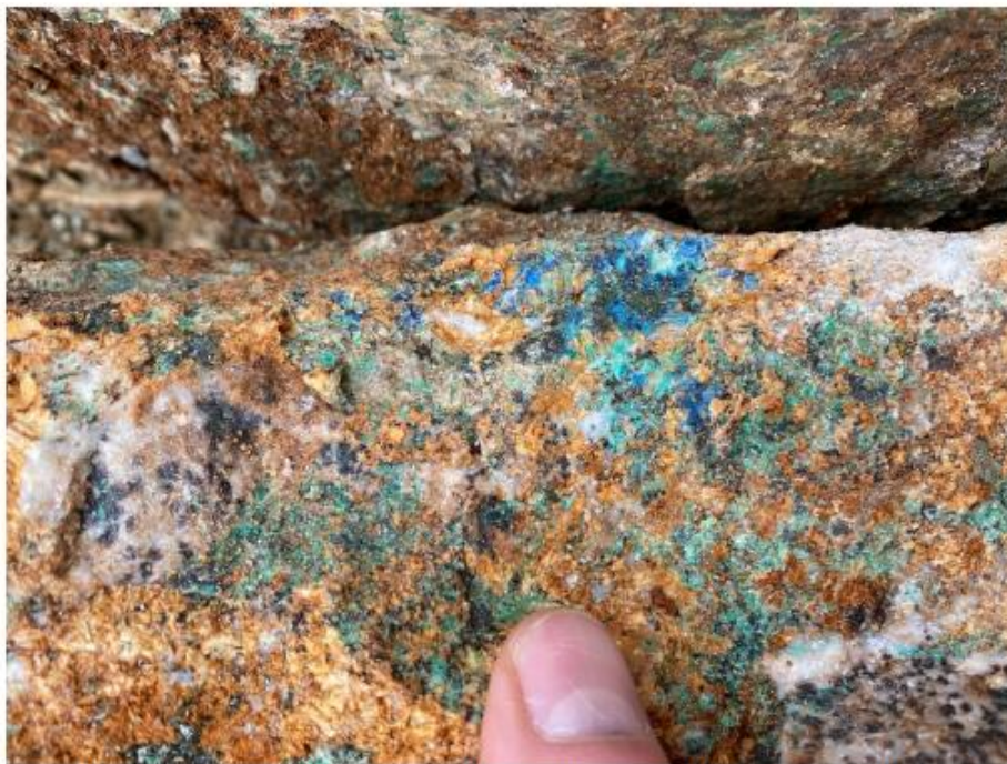
Figure 3. Characteristic chalcopyrite-chalcocite-malachite-azurite mineralization in quartz breccias the Cannon Zone.
