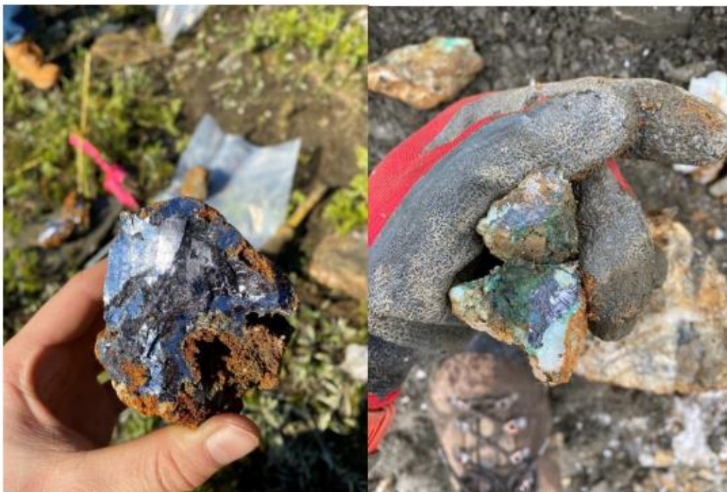
Figure 1. Mineralization present on the Gold Mountain Property. Left: oxidized botryoidal galena with malachite. Right: galena-chalcocite-malachite mineralization in a quartz-carbonate vein.
