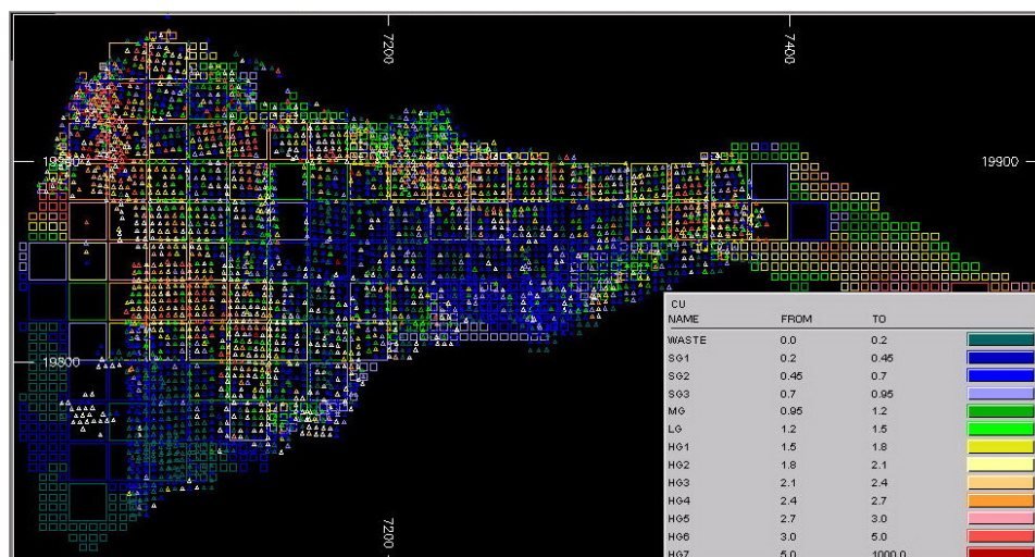
Figure 17.29 Horizontal plan view 1080m: comparison of estimated block copper grades with grade control drillhole composite grades
