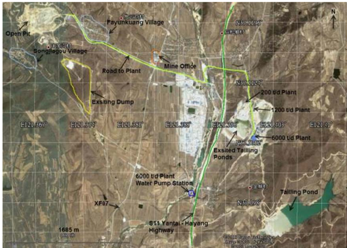
Figure 17-2: Mine Industrial Sites Lay-out
