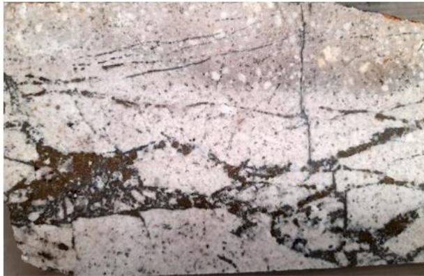
(a) (left): V2bx micro-veinlets dilating to form a local breccia zone. From AP-23-303 at 30 m depth.
