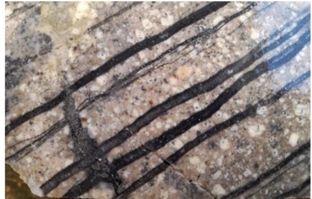
(a) (left): V2bx micro-veinlets dilating to form a local breccia zone. From AP-23-303 at 30 m depth.
