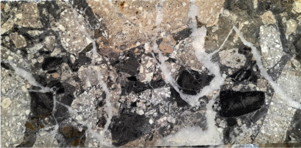
Polymictic Breccia illustrating late white quartz-calcite veinlets (V6qc) cutting across both clasts and matrix of the breccia. From AP23-297 at 83.4 m depth.
