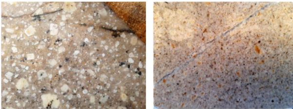
(a) (left): Feldspar porphyry with large plagioclase phenocrysts and minor disseminated fine grained pyrite from AP-23-291 at 17 m depth. (b) (right): Feldspar porphyry with small plagioclase phenocrysts and minor disseminated fine grained pyrite from AP-15-238 at 65 m depth.
