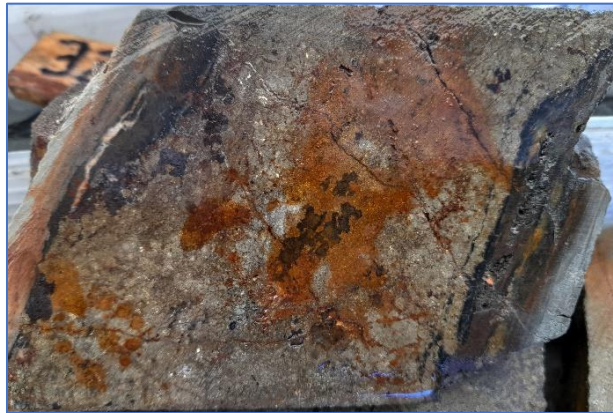
V3 patchy medium-grained pyrite overprinting the bedding of the sediments. From AP-15-238 at 33 m depth.
