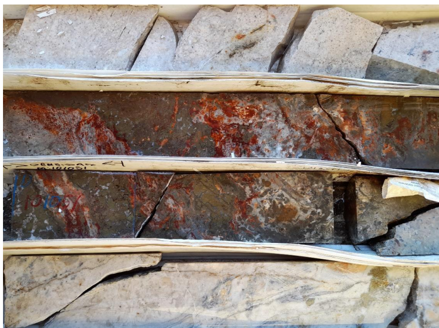
Figure 7-11: Thin Bedded Sediments Altered to Skarn (Photo 6)
