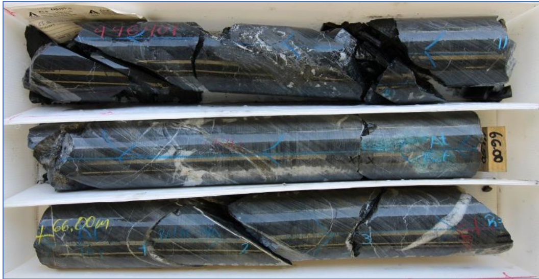
Thin bedded calcareous carbonaceous limestones and shales. From AP-23-299 at 66 m depth; PQ core so core width is approximately 8.5 cm.
