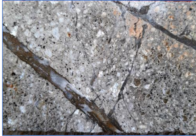
V2 micro-veinlets fractures (narrow diagonal veinlets) cut by V3 and V4 veinlets. From AP-23-291 at 147 m depth.
