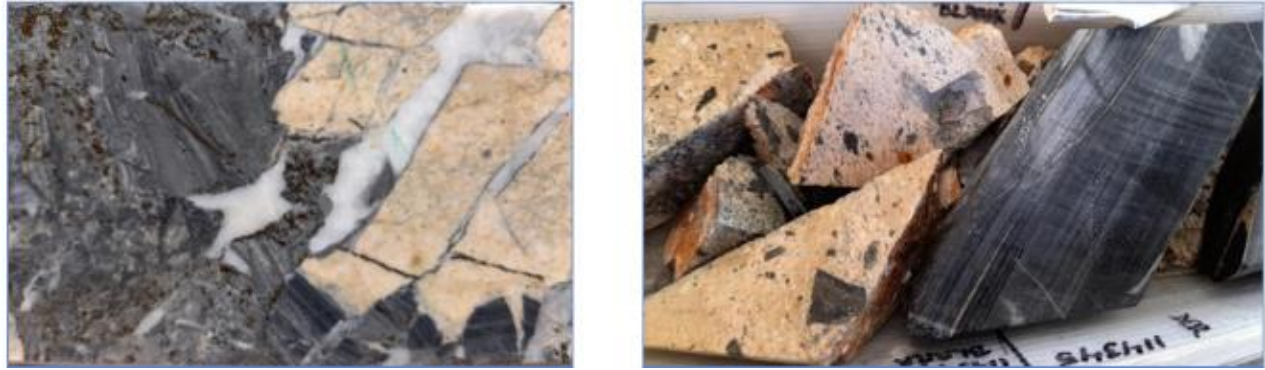
(a) (left): Contact Breccia showing crackle brecciation with feldspar porphyry clasts on the right and sediment clasts on the left. The white quartz veining is late epithermal overprint (V6q). From AP-11-76 at 304 m depth. (b) (right): Contact Breccia with a matrix of feldspar porphyry supporting sediment clasts. From AP-15- 238 at 28 m depth. Photos of HQ core with width of core of approximately 6.35 cm.
