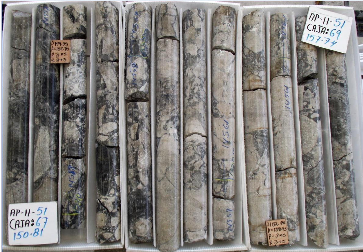
Monomictic Breccia with dominantly feldspar porphyry clasts with minor amounts of matrix, but note the polymictic clasts on the left side of the image. From AP-11-51 at 157.7 m depth; photo of HQ core with width of core of approximately 6.35 cm.
