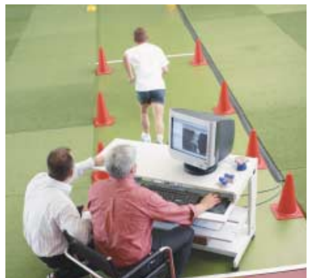
Rigorous biomechanical tests measure the shoe's shock-absorbing system and the effects on the runner's body.
