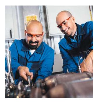
At BASF Catalysts' testing facility in Union, New Jersey, technician David Colon (left) and Andrew Thoms set up a catalyst test on the motor testing bench. In the engine laboratory, catalysts are subjected to long-term stress testing. Modern testing technology makes it possible to simulate three-way-catalyst durability (120,000 miles of catalyst activity) in 50-100 hours.
