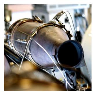
Vehicle catalysts are tested under long-term conditions at BASF's catalyst testing facility in Union, New Jersey. Complex electronic sensors are used to record all exhaust gas values during testing. The experts at BASF Catalysts are among the leading innovators in the development and optimization of catalysts for gasoline and diesel engines.
