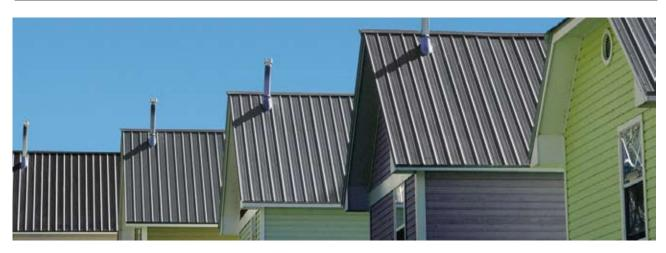
NEW SOLAR REFLECTING PIGMENTS FROM BASF are used, for example, as the basis for roof coatings. The pigments prevent heat absorption so energy consumption is lower in summer. They also extend the lifetime of the roof.
