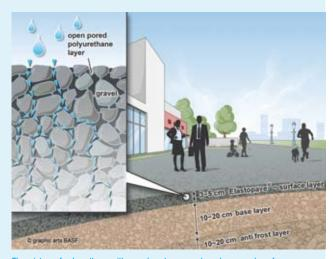
The mixture of polyurethane with gravel or stones creates a large number of connected cavities in the Elastopave surface so the ground is not sealed and water can flow through.
