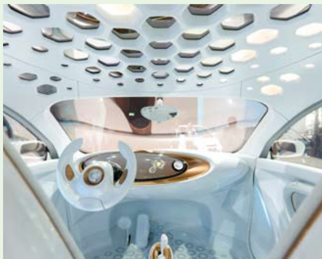
Organic light-emitting diodes illuminate the vehicle interior in the dark. They are transparent, creating a sunroof effect during the day.
