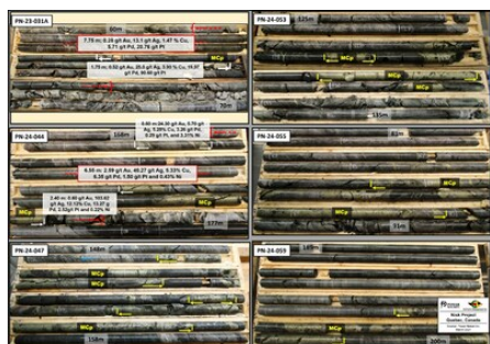
Figure 3: Core pictures showing the relation between observed massive chalcopyrite and grade in both PN-23-031A and PN-24-044, and massive chalcopyrite (MCp) observed in four other recent holes. (CNW Group/Power Nickel Inc.)
