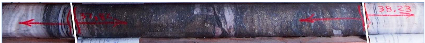
Drill Hole A-J 21-03 core (37.82m-38.23m) 20.5 g/t Au over 0.41 metres
