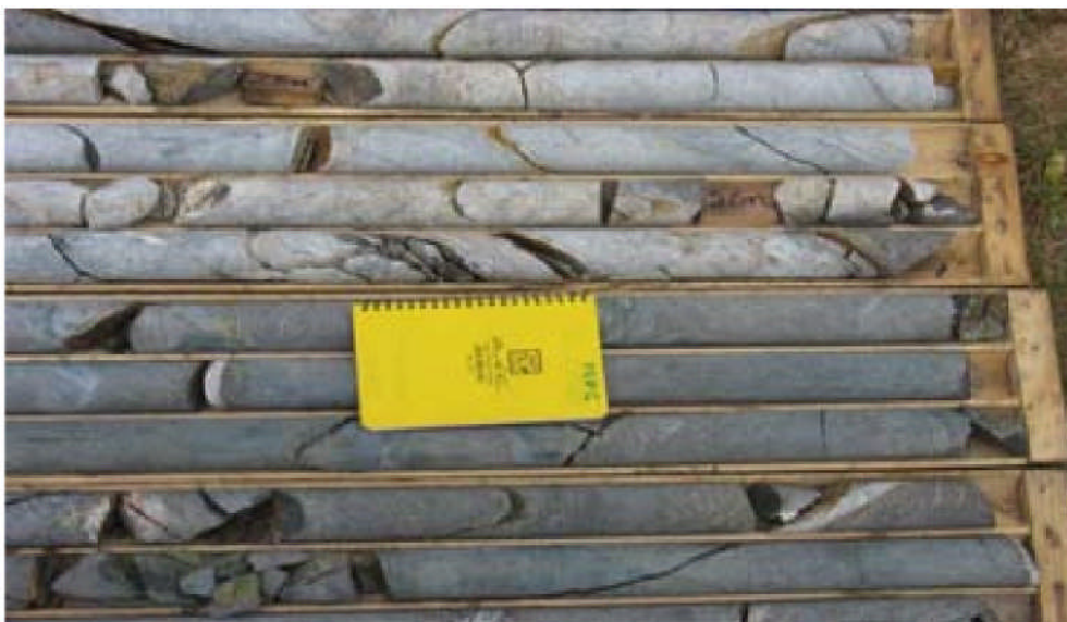
Figure 10.2 Altered feldspar porphyry and gabbro with disseminated sheelite in gabbro indicated by yellow pencil marks (Drill hole SB06-14)
