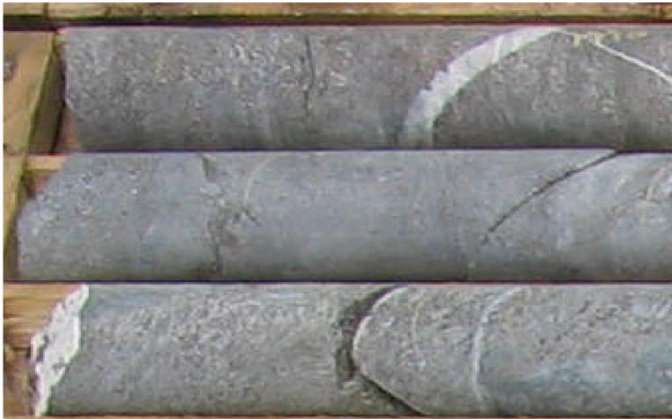
Figure 10.2 Altered feldspar porphyry and gabbro with disseminated sheelite in gabbro indicated by yellow pencil marks (Drill hole SB06-14)
