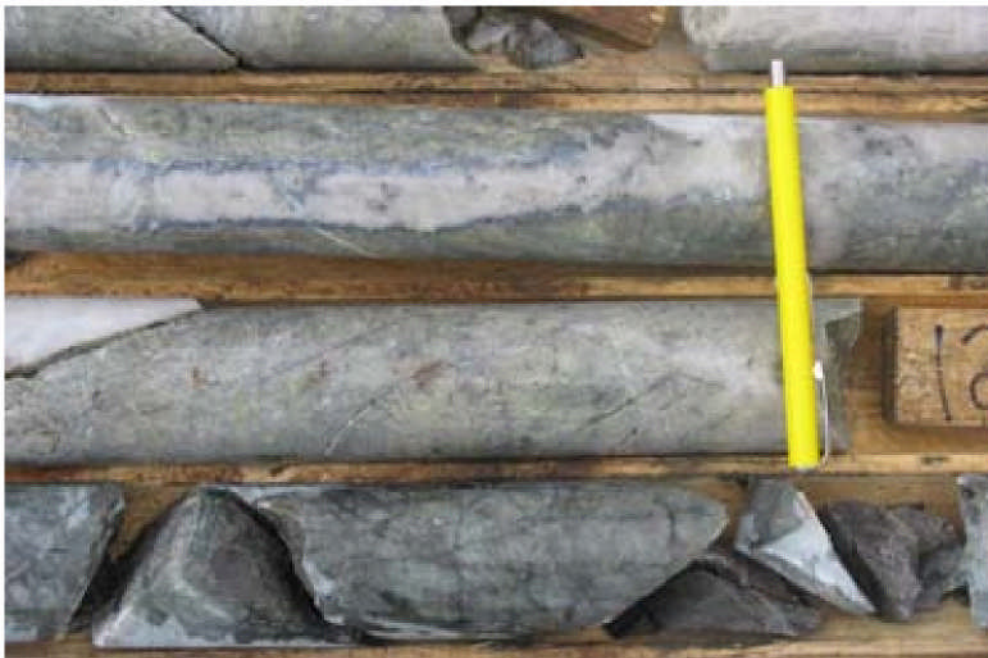
Figure 10.4 Altered felsic tuff with molybdenite in quartz vein (Drill hole SB06-14)
