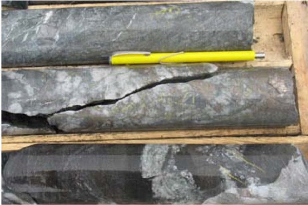
Figure 10.4 Altered felsic tuff with molybdenite in quartz vein (Drill hole SB06-14)
