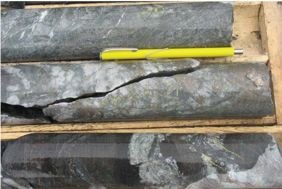
Figure 7: Altered mafic tuff with pyrrhotite, chalcopyrite and scheelite (yellow pencil marking) in quartz veining (Drill hole SB06-14)
