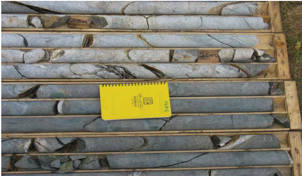
Figure 6: Altered feldspar porphyry and gabbro with disseminated scheelite in gabbro indicated by yellow pencil marks (Hole SB06-14)
