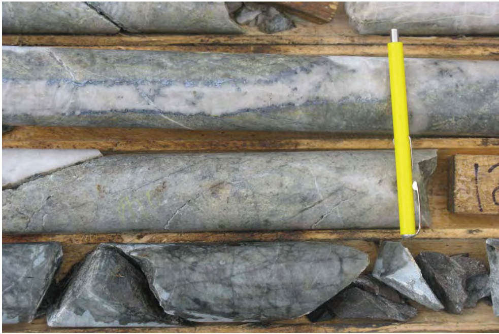
Figure 8: Altered felsic tuff with molybdenite in quartz vein (Drill hole SB06-14)
