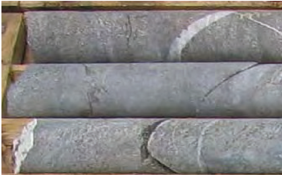
Figure 5: Altered gabbro with chloritized amphibole alteration and quartz veining (Hole SB06-14)
