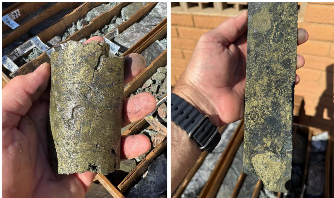
Photos 1 & 2: High-grade replacement style massive sulphide mineralization intercepted in CC24-026 consisting of massive pyrite and chalcopyrite hosted in the favourable Abrigo Formation.
