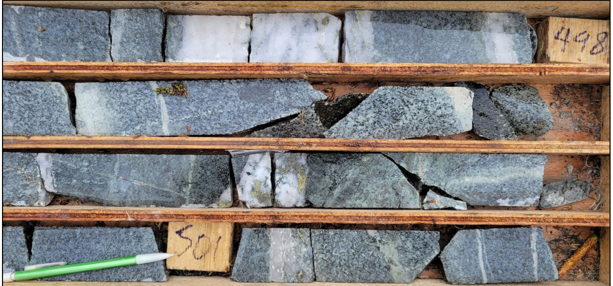
Figure 2: Porphyry-style quartz-sulphide and sulphide veining, associated with weak phyllic alteration overprinting propylitic alteration within the granodiorite intrusion. Photo is from LIB24-004 between 497.5 m and 501.3 m.
