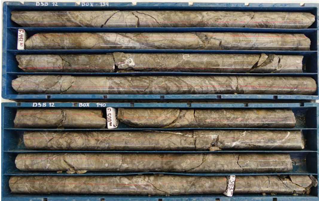
Figure 3: Pictures of Diamond Drill Core Samples from Hole DSB-12
