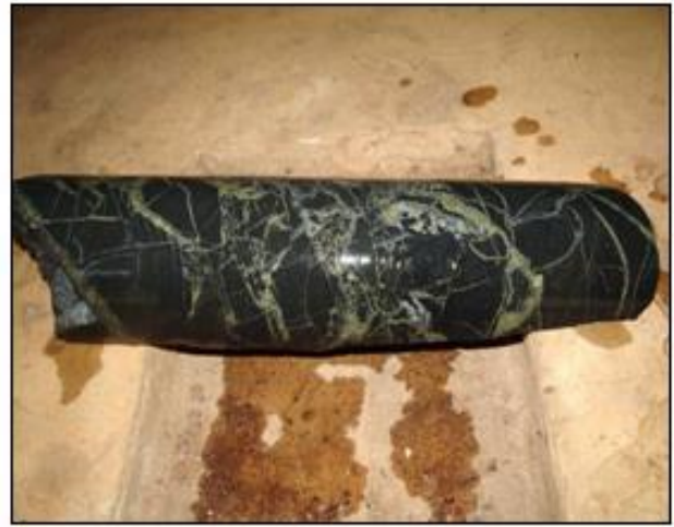
Figure 3. High grade oxide drill core Kasala Project & Sulfide drill core at depth on Kasala
