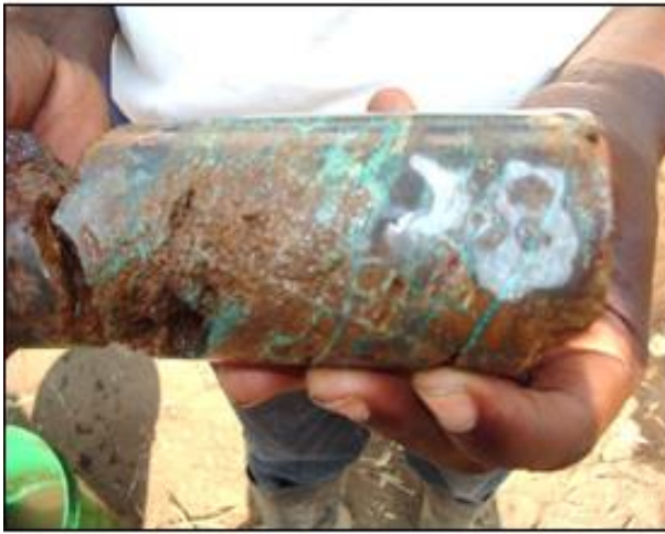
Figure 3. High grade oxide drill core Kasala Project & Sulfide drill core at depth on Kasala
