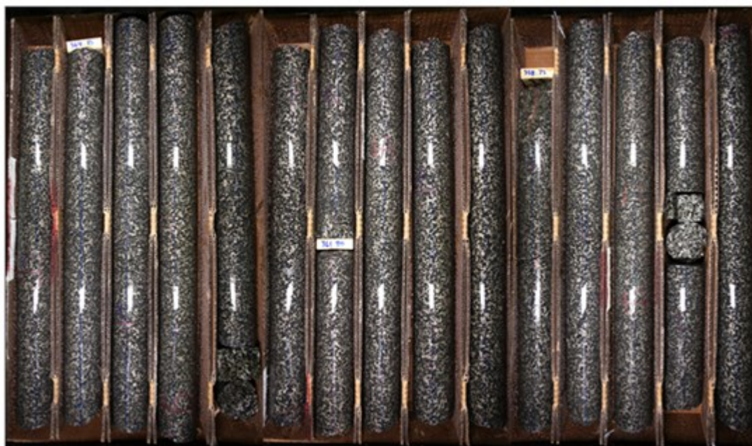
Figure 1: Portion of Drill Hole 20TK0277 representing 39 meters (128 feet) of semi-massive sulphide mineralization grading 3.12% Ni, 1.60% Cu, 0.08% Co, 0.13 g/t Pd, 0.21 g/t Pt and 0.17 g/t Au (3.94% NiEq or 10.51% CuEq) starting at 346 meters
