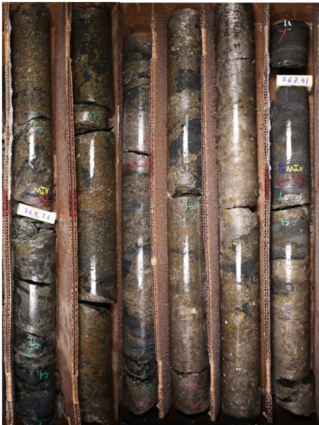
Figure 1: Drill hole 21TK0358 assayed 5.65% Ni, 2.04% Cu (6.88% NiEq, 18.36% CuEq) over 2.93 meters starting at 264.3 meters depth
