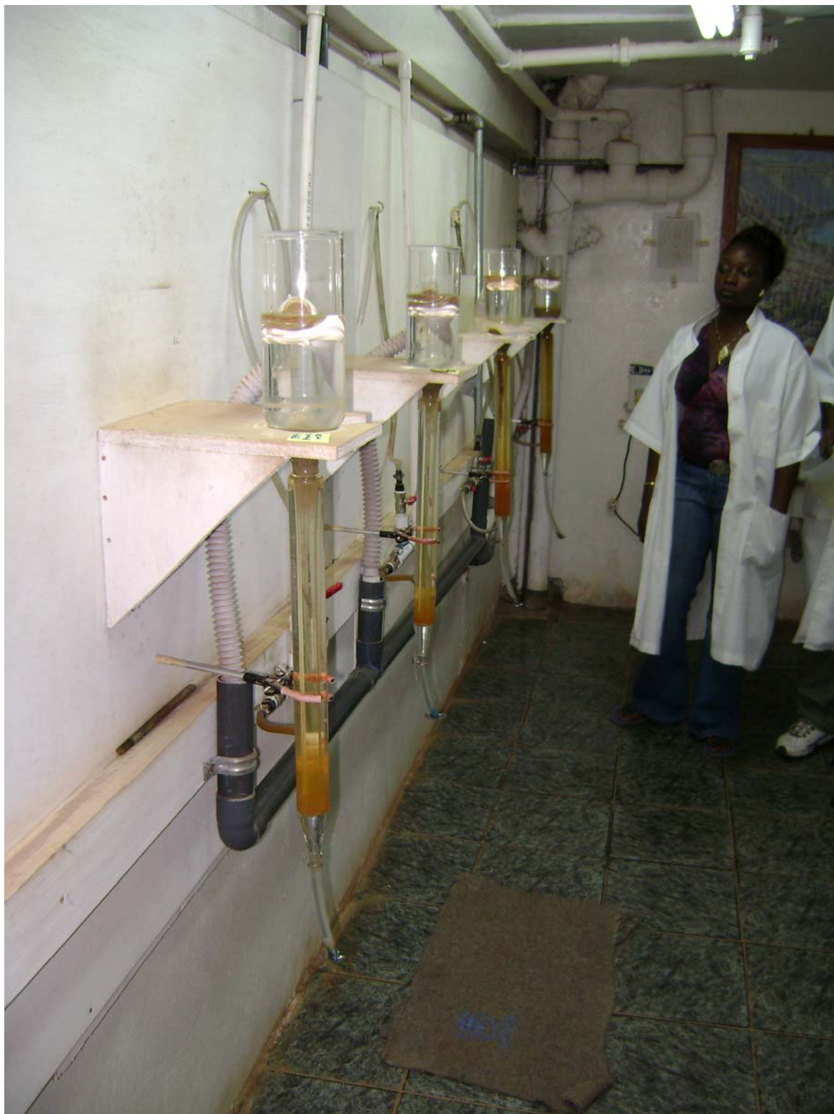
Photo 18 Water Columns for Concentration of Heavy Minerals, WMRC Laboratory, Monrovia
