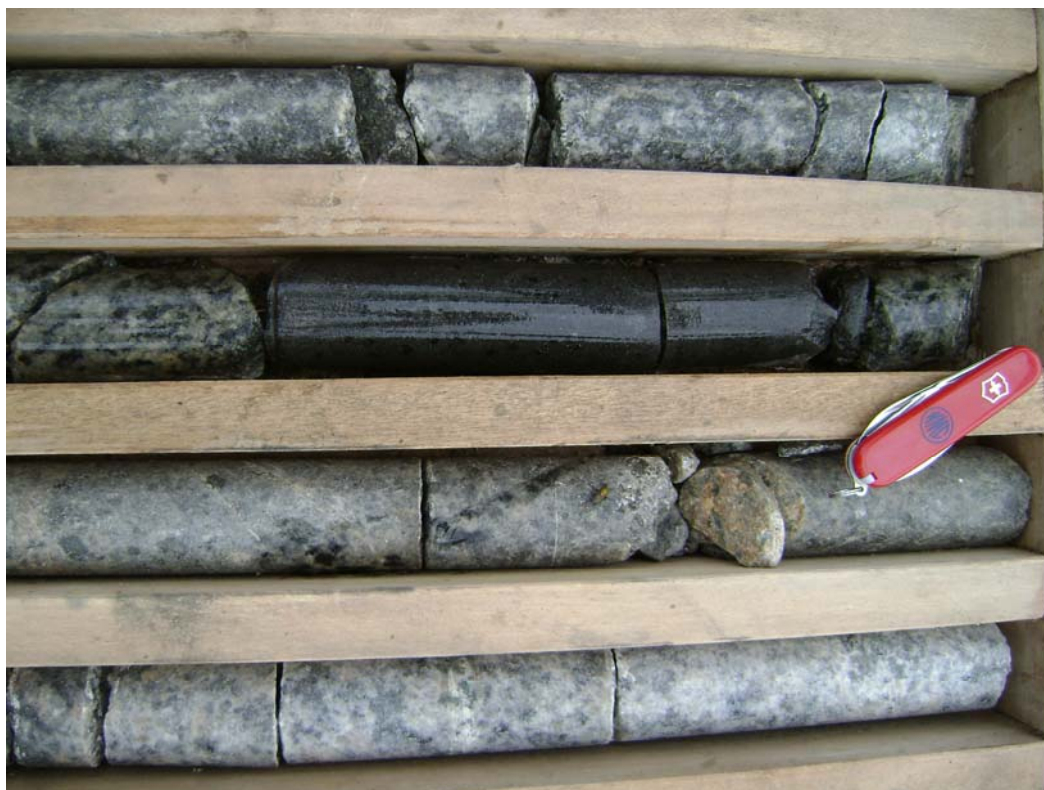
Photo 8 Kimberlite Intersection, Tongo, Probably Vein Parallel to Tongo 1 Dyke
