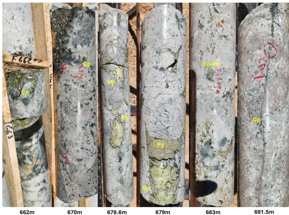
Figure 3. Examples of mineralization observed in hole FZ-DH-25-68. Cp: chalcopyrite; Py: pyrite. HQ core (63.5mm)
