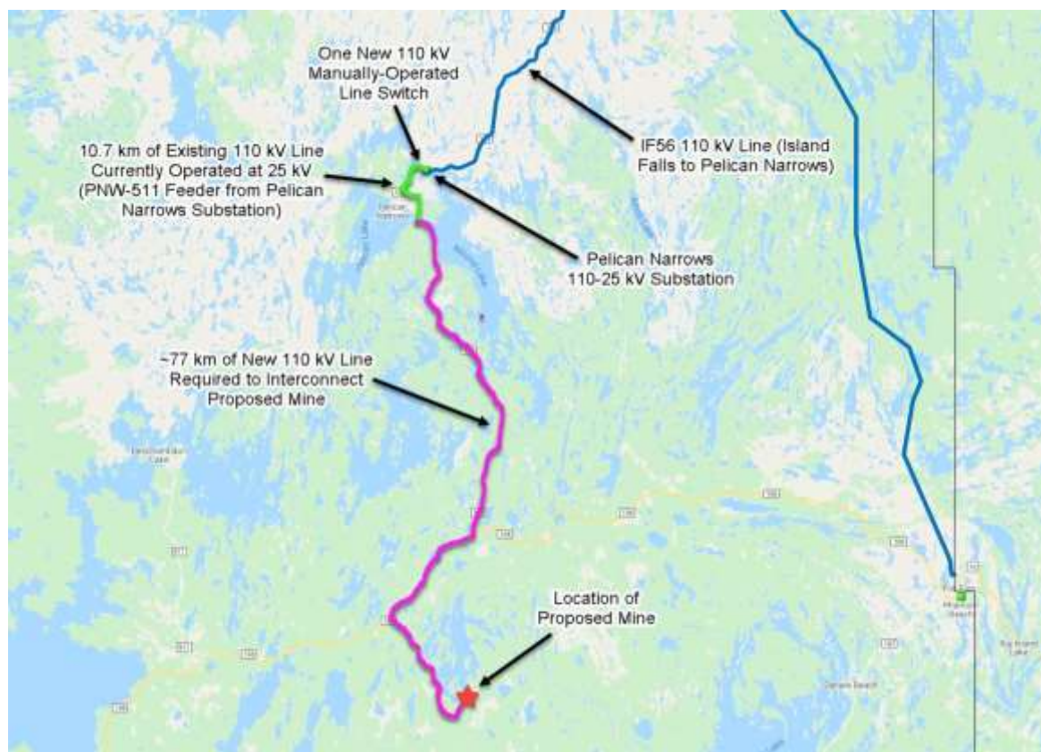
Figure 18-10: Proposed 138 kV SaskPower Transmission Line (SaskPower, 2021)
