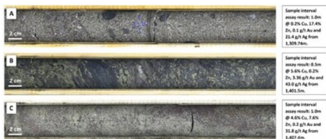
Figure 3. Photo examples and associated assays of lenses in TS-25-37 A) Clastic pyrite and interstitial sphalerite Zn-rich massive sulphide (1,310m); B) Chalcopyrite-rich, gold bearing copper stockwork zone hosted within felsic volcanics (1,401.5m); C) Interval of massive sulphide hosting significant sphalerite and chalcopyrite (1,407.4m) (CNW Group/Foran Mining Corporation)
