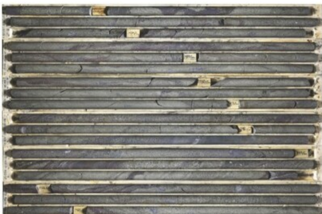
Figure 5 – Example of the massive to semi-massive sulphide intersection described for TS-25-37w1 (1,401.1 - 1,426.7m). Assays are currently pending for this hole and further analysis is required to confirm the significance of any mineralization therein. (CNW Group/Foran Mining Corporation)
