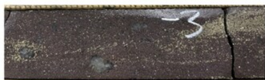
TS-25-37W1 - 1430.9m - Sphalerite and Pyrite 0.74m @ 0.04% Cu, 32.0% Zn, 6.9 g/t Ag and 0.06 g/t Au
