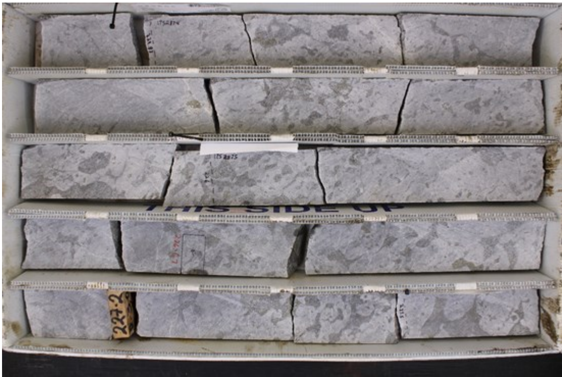
Figure 3: Drill core from B21C-016 at 227m depth showing distinct patchy pyrophyllite (aka "gusano") alteration textures
